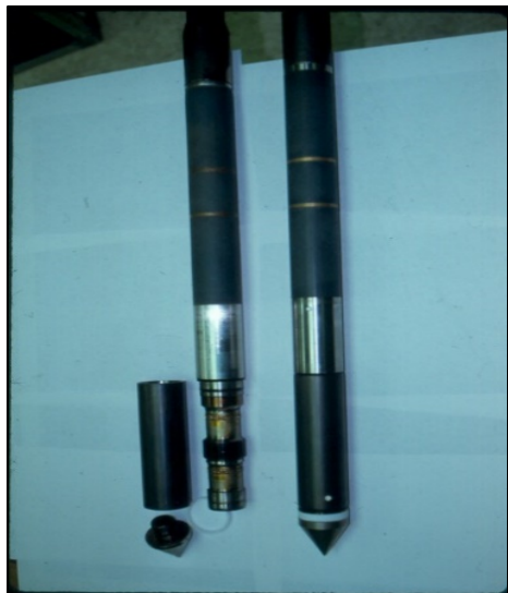
Image 2. Cone Penetrometer
