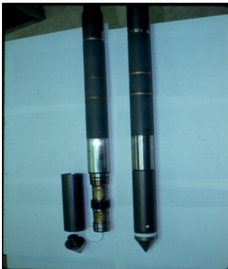
Image 2. Cone Penetrometer
