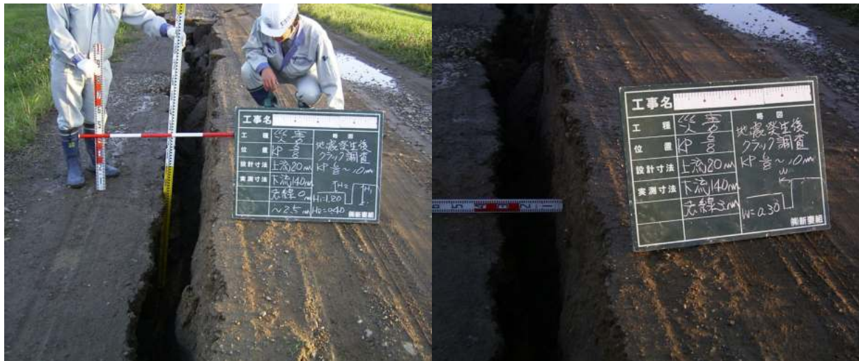
Figure 4.14 Cracks and differential settlement on the crest access road at Section 7.
