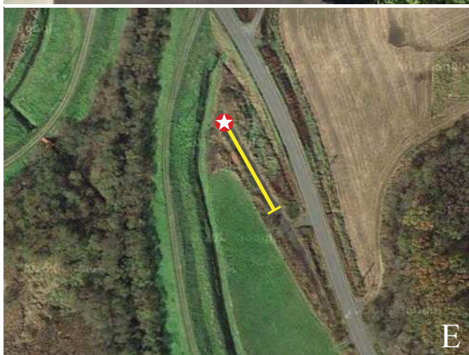
Surface wave test site 1054HK located outside the Urahoro left bank levee, location L -0.2, 41 km SE of (lat 42.743, long 143.67023). A) view southeast from the shaker to the seismometer array; B) view north at the shaker location; C) another view southeast from the shaker; D) site information; E) satellite view of the local site, yellow bar is seismometer array; F) site location near Obihiro, Hokkaido, Japan.
