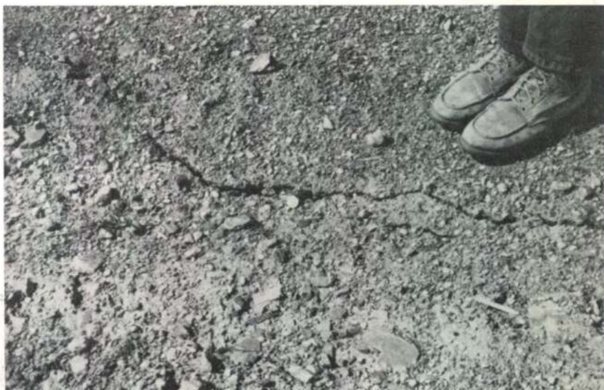
View of a pre-existing crack on Venice Island (Site 15) that lengthened 50 feet and dropped 2 inches during the April 24, 1984 Morgan Hill earthquake. Photograph taken the day after the earthquake.
