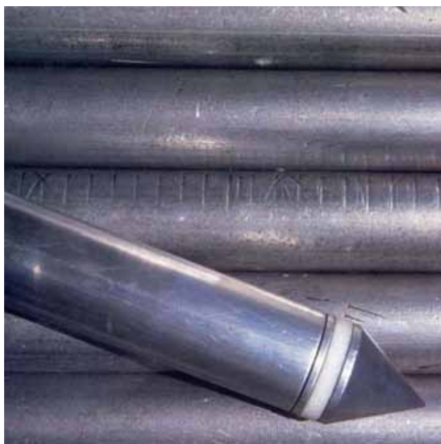
Figure 11–1 Working end of cone penetrometer ( Photo courtesy of Gregg Drilling & Testing, Inc. )
