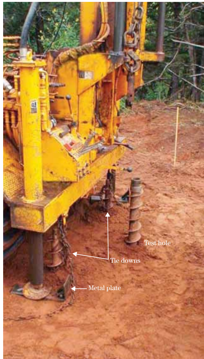
Figure 11-6 Drill rig set up to conduct SCPT. Metal plates are struck with a sledge hammer to initiate energy pulse. The seismic cone penetrometer has a geophone incorporated into its design. (Photo courtesy of Glen Miller, Geologist (retired), NRCS, Stillwater, Oklahoma)
