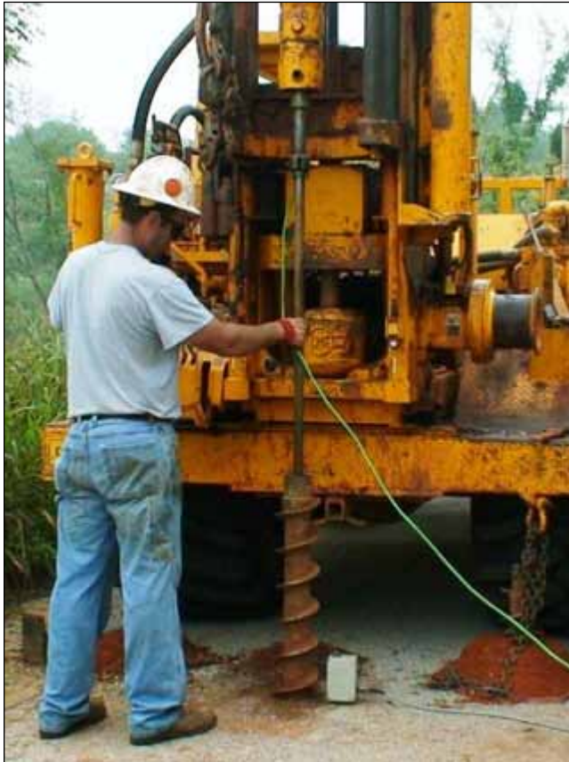
Figure 11-7 SCPT being conducted through hollow stem augers (Photo courtesy of Glen Miller, Geologist (retired), NRCS, Stillwater, Oklahoma)
